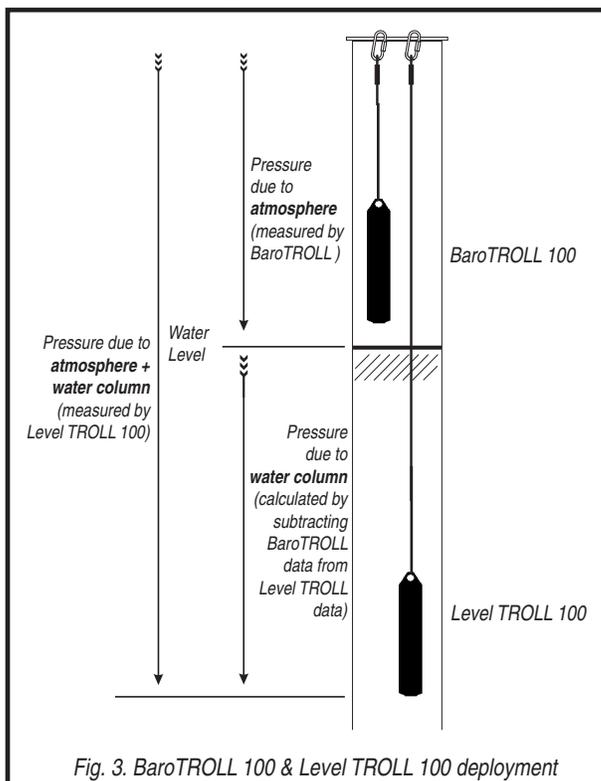
Fig. 3. BaroTROLL 100 & Level TROLL 100 deployment
