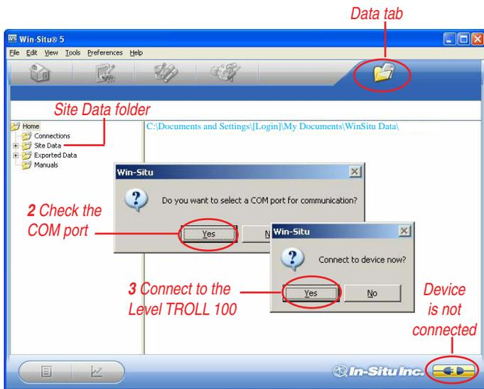
Fig. 1. Win-Situ Data tab on first connection
